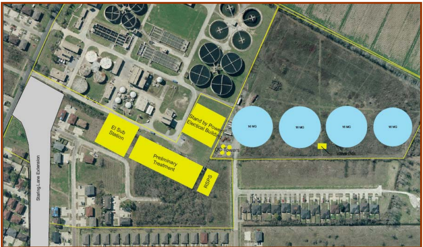
Proposed site layout for the South Wastewater Treatment Plant Wet Weather Improvements Project
