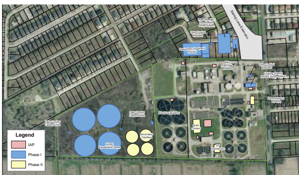
A geotechnical investigation was conducted to determine the feasibility of constructing the four new Flow Equalization Tanks that will be used to hold 16 Million Gallons of wastewater before being treated.
