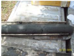
Geotechnical Engineers are drilling soil samples in the Northwest Area of the SWWTP. Results of the soil samples will be used to help assess the site characteristics where the proposed Equalization Tanks will be constructed.
