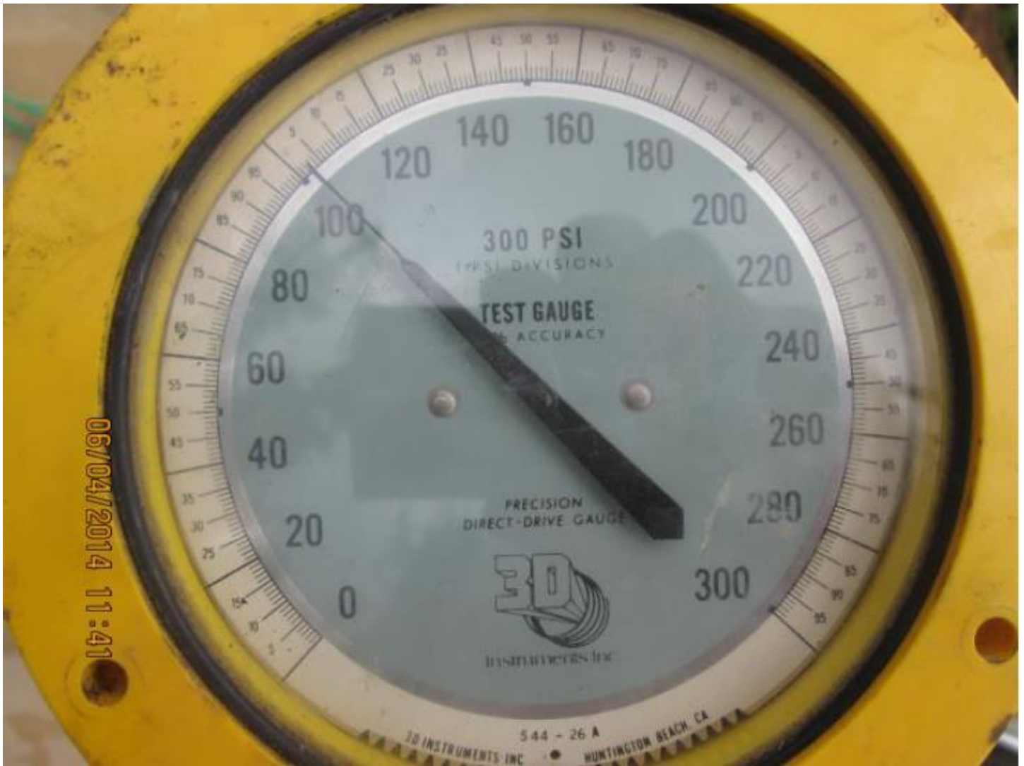
Figure 7. Test gauge during forcemain testing
